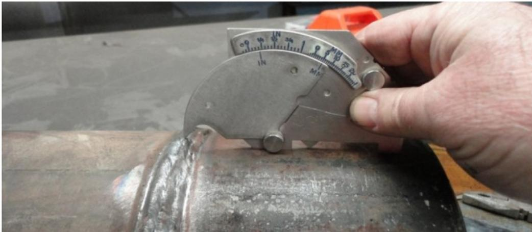
Direct visual inspection applies proper lighting, measurement, and comparative tools with the experience of our qualified technicians to determine design compliance and conformance to drawings, codes and specification requirements [E.g. AWS D1.1, BS EN 1370, BS EN ISO 17637, ASME B31.1, ASME B31.3, ASME Section VIII Div. 1, ASTM A802, ASTM A997, etc.].
