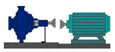
Vibration Analysis is mainly used in the detection of the rotating equipment problems like imbalance, bent shaft, misalignment, soft foot, looseness through the study of the vibration coming from the equipment due to the problems. It is used to study Bearing problems, Gear Box Problems, etc.
