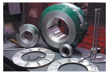
Typical types of composite white metal bearings include integral or split journal and thrust bearings with fixed profile as well as journal and thrust pads. In this context, composite white metal bearings also include non-contacting seals, oil supply casings, sliding and guiding elements with similar design features.
