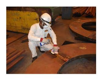
TOMTEC performs both visible and fluorescent liquid penetrant testing in accordance with ASTM E1417, ASTM E165, ASTM E1418, ASTM E433, ASTM E1209, ASTM E1219, ASTM E1220, ASME BPVC Section V - Article 6, EN 571-1 and similar national and international standards.
