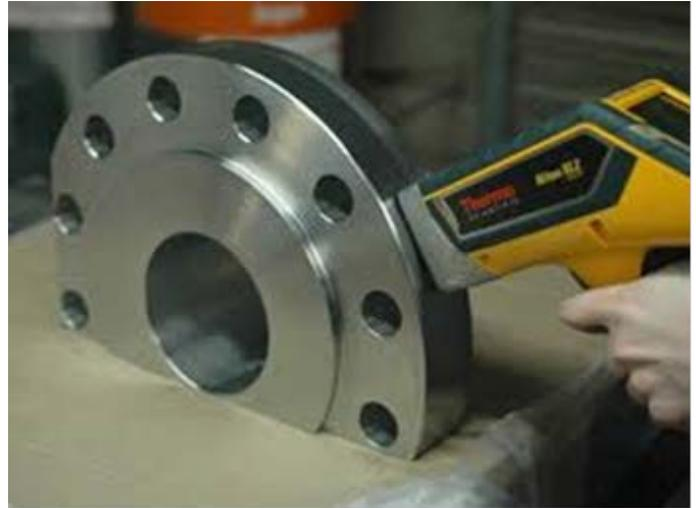
Typical methods for PMI include X-ray fluorescence (XRF) and optical emission spectrometry (OES). TOMTEC carries out PMI using the latest portable analyzers. Test results are summarized in an inspection report.
