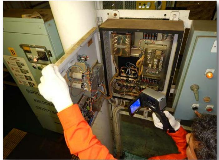
Without shutting down the equipment, or interfering with production, a thermographic inspection can detect problems in electrical panels, motor control centers, switchgear cabinets, disconnects, transformer bushings and terminations, and equipment control panels that may result in electrical fires, mechanical breakdowns, or significant business interruption.
