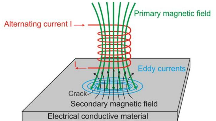
At TOMTEC, our skilled technicians are experienced in this method, have internationally recognized qualifications and onsite experience. TOMTEC Performs test in accordance with BS EN ISO 17643, ASME BPVC Section V – Article 8, ASTM E376, ASTM E566, ASTM E703, ASTM E1004 and similar National and International Standards.
